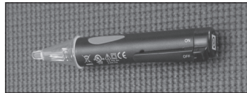
Use a non-contact circuit tester to check for electrical power.
