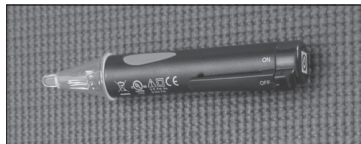
Figure 2 - Use a non-contact circuit tester to insure that the power is off before you work on a circuit.
