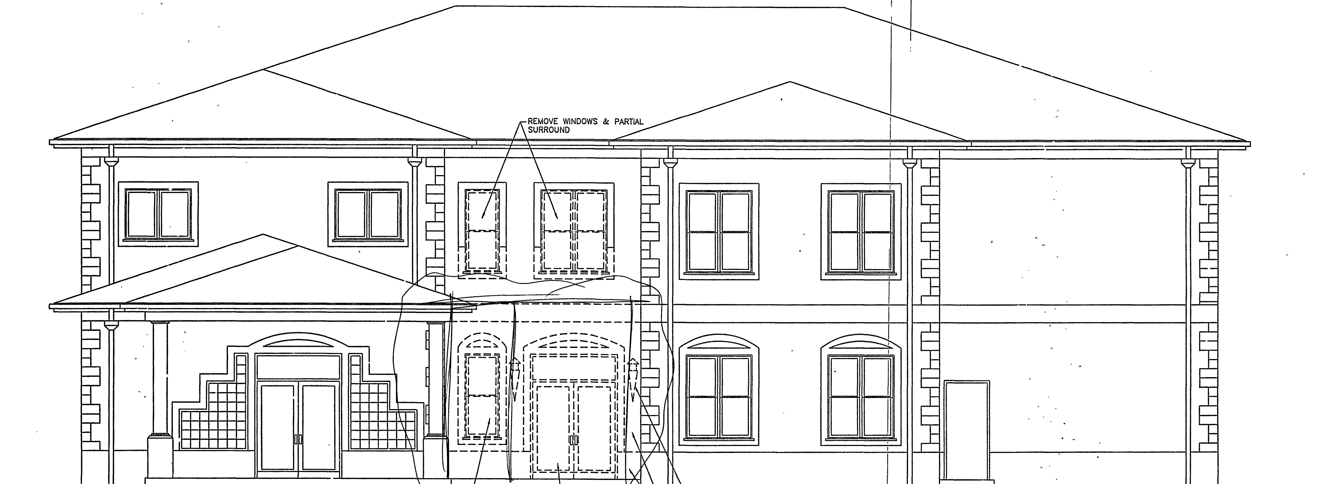
A NORTH ELEVATION: AS-BUILT / DEMO A-4 1/4" = 1'-0"
