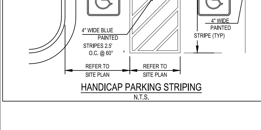
HANDICAP PARKING STRIPING N.T.S.
