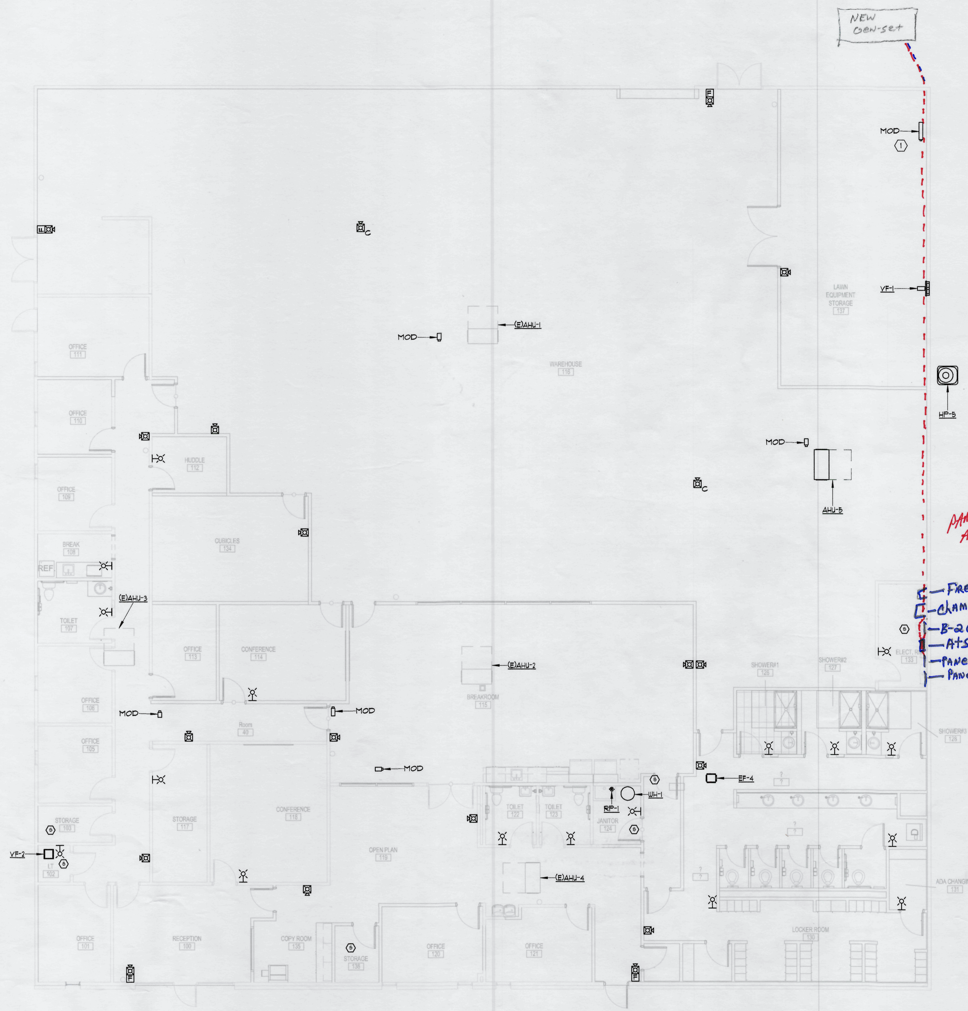
FLOOR PLAN - MECHANICAL AND FIRE ALARM 1/8" = 1'-0" NORTH KEY NOTES: ① CIRCUIT NEW M.O.D. TO NEAREST CONVENIENCE RECEPTACLE CIRCUIT. (TYPICAL)
